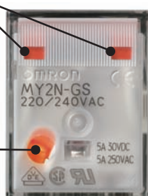
Relay with AC Coil (LED: Red)
