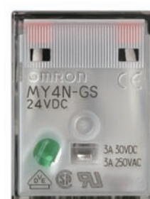
Relay with DC Coil (LED: Green)
